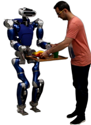
Fig. 1. The humanoid robot TORO transporting objects on a tray.
